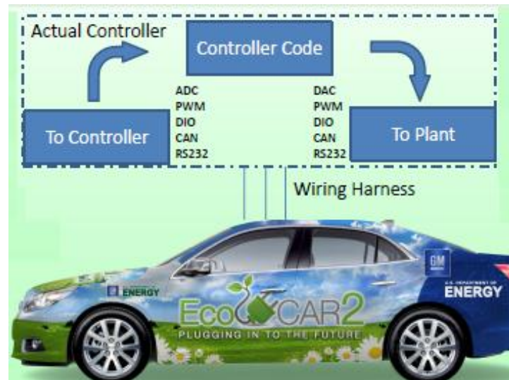
Figure 1-4. VIL (Vehicle-in-the-loop) Data Flow [9]
